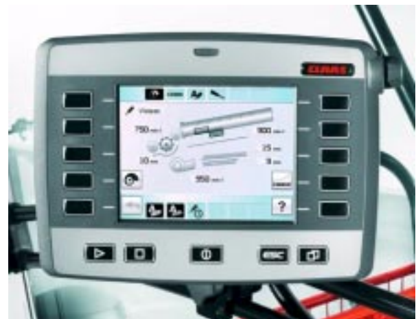
Claas Cemos control unit for Lexion 700 farm combines
